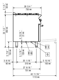
Electrical inlet (power) Gas connection
