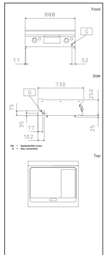
Gas Power: 14 kW Gas Type Option: LPG Gas Inlet: 1/2"
