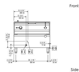
CWI1 = Cold Water inlet 1 EI = Electrical inlet (power)
