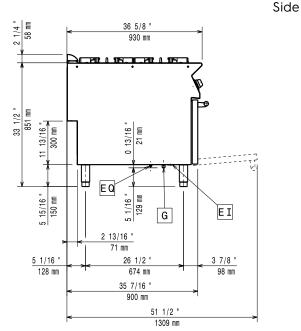
Electrical inlet (power) Gas connection
